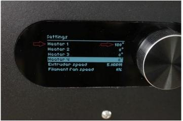
Press "Start extrusion" and select "Manually" (this ensures the screw will not start after reaching the target temperature).
