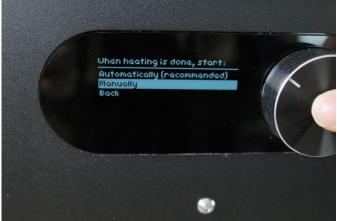
Set the timeout to 4 minutes, and click 'OK', the system starts heating. After the timeout, the heaters will turn off and the system will cool down slowly, you will have plenty of time to replace the nozzle.
