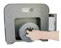
Place spool holder on winder by sliding the metal rod into the tube.
