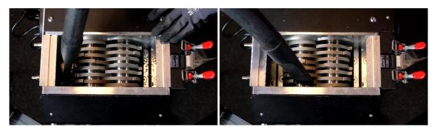
15. Vacuum the shredder combs one by one. If necessary, use a clean brush to get in between the teeth of the combs.
