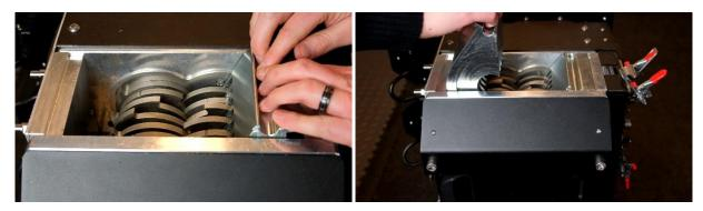
21. Insert granulator filter by sliding it into the machine.
