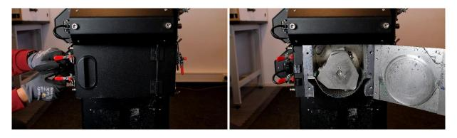
12. Remove filter screen by sliding it out of the machine, towards you. Place on side.
