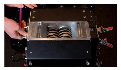
10. Remove shredder combs, and place safely on side.
