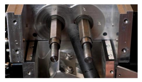
10. Brush off or wipe each blade. Careful with the edges as they can cut. Wear cutproof gloves, if necessary.
