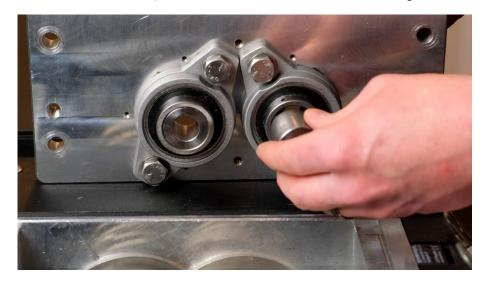
22. Slide the plate onto the two axles, careful not to let the bearings fall out.
