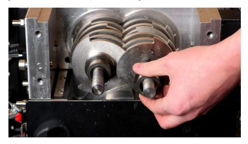
8. Slide off each blade and spacer one by one. It helps to pile them in two stacks without changing their direction.
