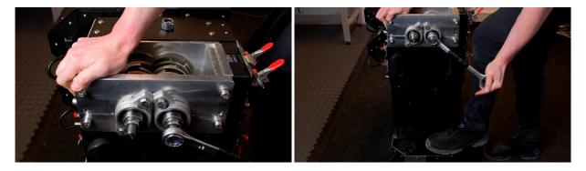
26. Attach the cover plate and add a small amount of blue Loctite to each bolt, before screwing them and tightening them thoroughly.
