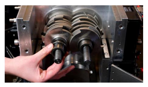
21. On a flat surface, hold the side plate and insert the two round bearings into the two holes.
