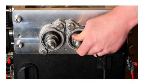
4. Loosen 4 bolts in the corners of the shredder side plate. The plate will stay secure on the axels. Place on the side.
