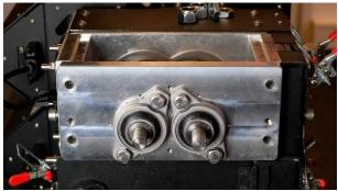
5. Slide off the side plate, and place on the side.
