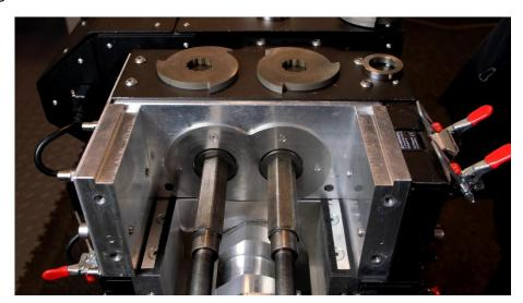
II. The blades and spacers alternate on a single axle: blade, spacer, blade, spacer etc. And the blades alternate on the two opposing axles, as illustrated below.
