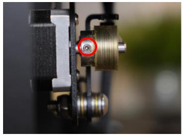
**Step 4:** When the set screw is removed the puller wheel can be removed by sliding it away from the Filament Maker while also pushing down on the lever. This is presented in the pictures below.
