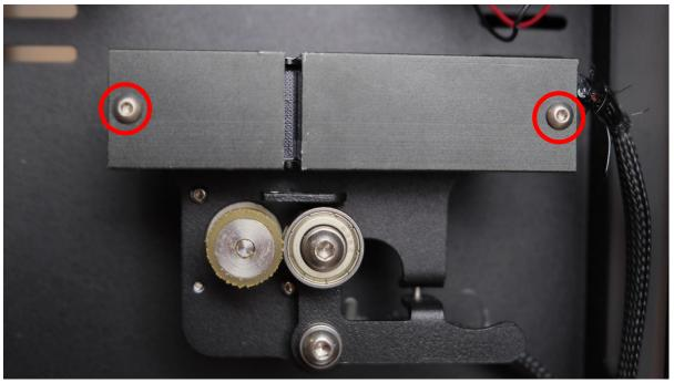
**Step 2:** After removing the bolts place the sensor carefully at the bottom of the Filament Maker without putting tension on the wire that connects the sensor to the Filament Maker. This is also presented in the picture below.
