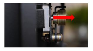
**Step 5 (optional):** In very special cases the puller wheel can be very difficult to slide of the puller wheel as it is tightly mounted on the Filament Maker. In these cases a pulley puller such as presented below can be used.
