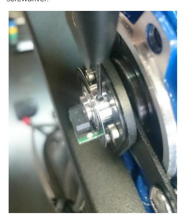
Step 11: Carefully remove the encoder sensor.
