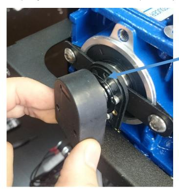
Step 9: Unscrew the two bolts on encoder sensor.
