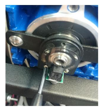
Step 17: Make sure that the encoder wheel is as much in the middle of the gap in the encoder sensor as possible before you fasten the setscrew.
