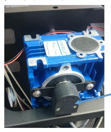
Step 7: Use the #1 Phillips screwdriver to unscrew the two bolts on front of the encoder
