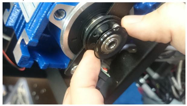
Step 15: The encoder sensor can now be placed back on its place. You can either place the encoder sensor simultaneous with the encoder wheel or afterwards.
