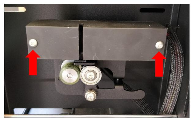
Step 4: Gently push the inside frame of the filament sensor out of the tube from the side <u>without</u> cables.
