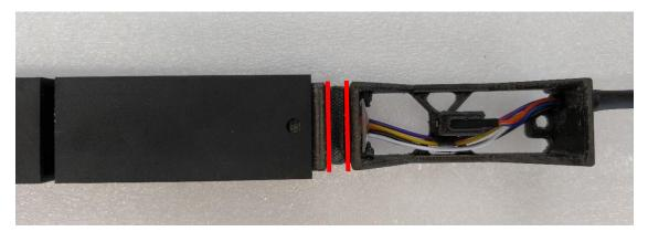
Step 6: Gently slide the inside frame of the filament sensor back in the tube. While sliding, check the corners highlighted underneath to make sure everything fits properly.
