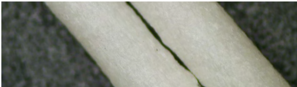
Figure 7 - Microscope shot to show the visual aspect of the filament : smooth, homogeneous, clear, consistent
