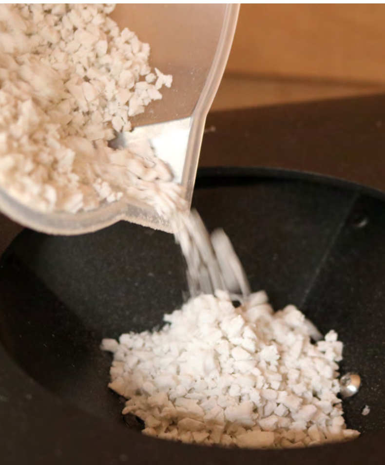
Figure 2 - Feeding FS92 regrind into the hopper of the extruder
