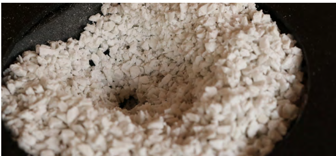
Figure 5 - Ratholing in the hopper
