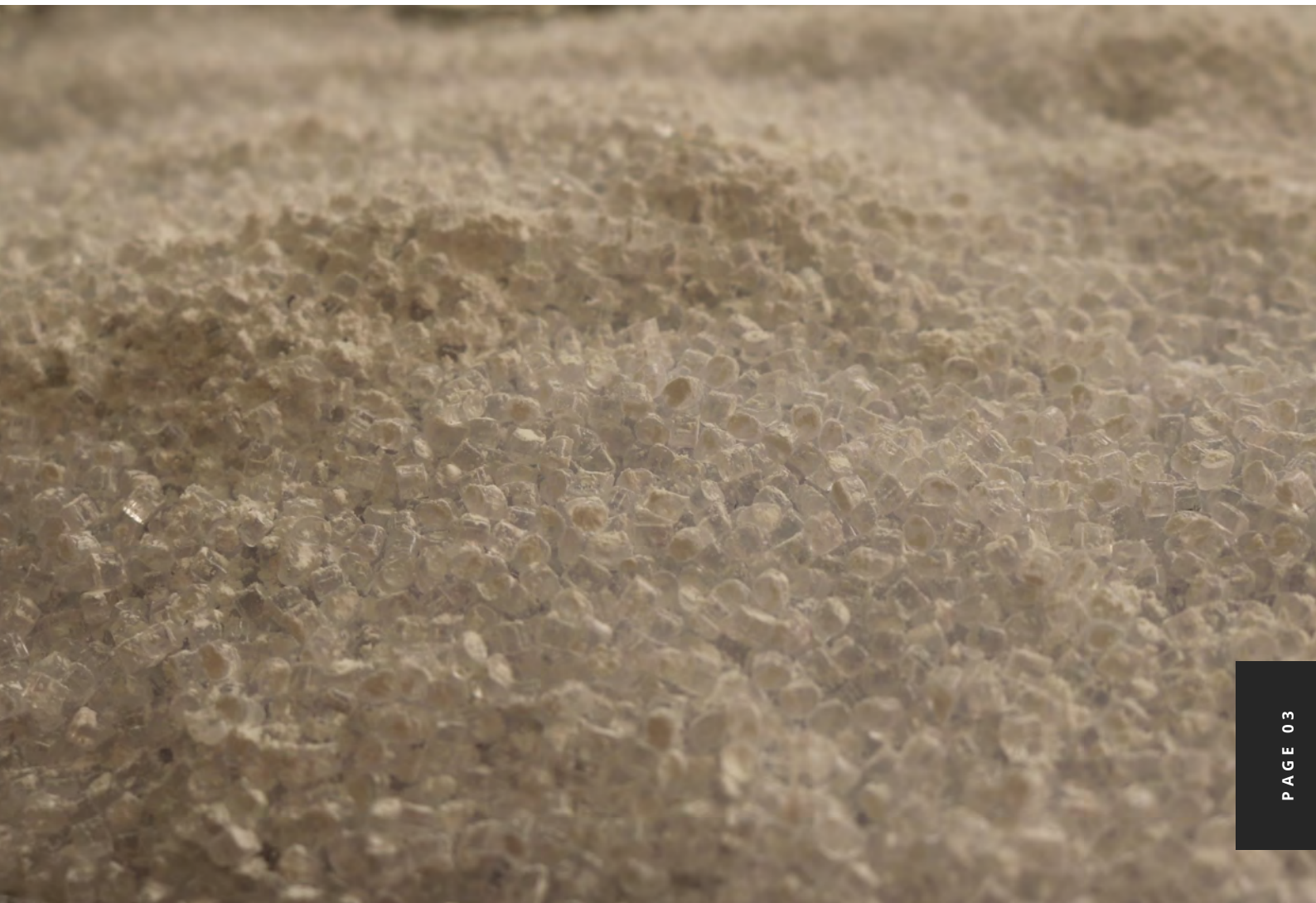
Figure 1 - Pellets of PC (transparent) mixed with PTFE powder (white)
