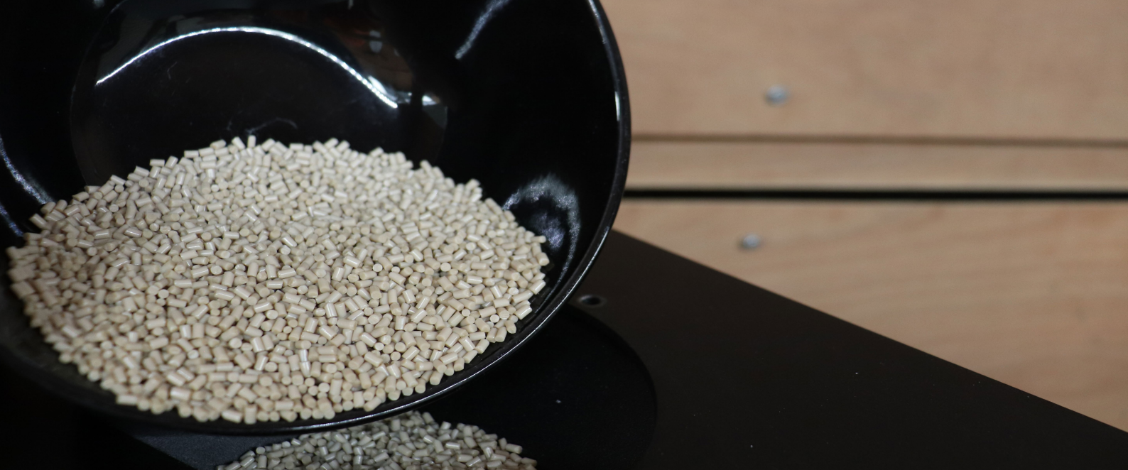
Figure 3 - Feeding PEEK into the hopper of the extruder
