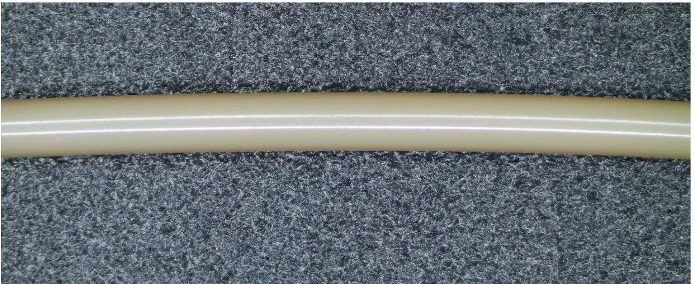
Figure 6 - Microscope shot to show the visual aspect of the PEEK filament : smooth, homogeneous, consistent
