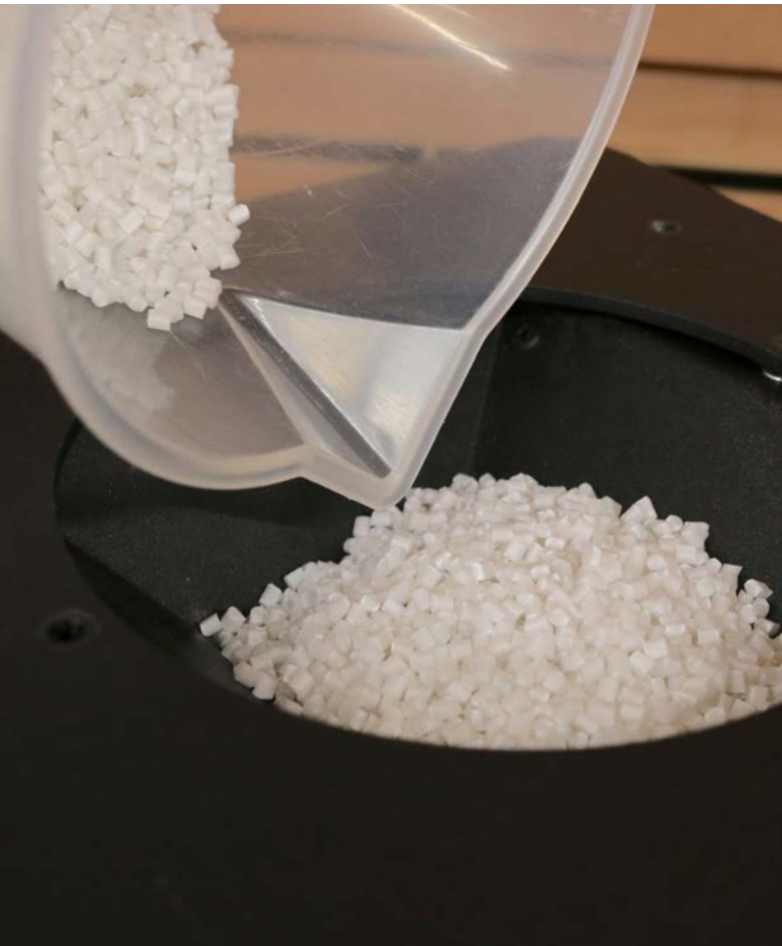
Figure 2 - Feeding PP pellets into the hopper of the extruder
