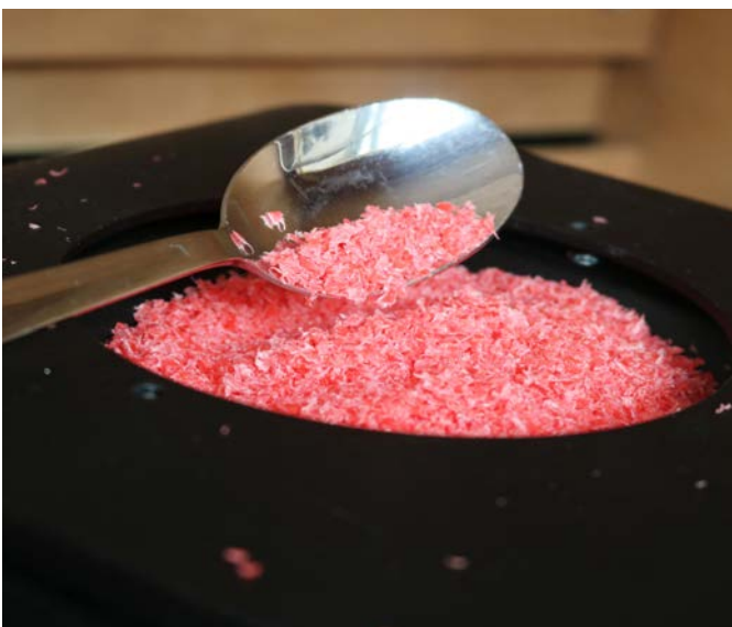
Figure 8 - Feeding LLDPE regrind into the hopper of the extruder
