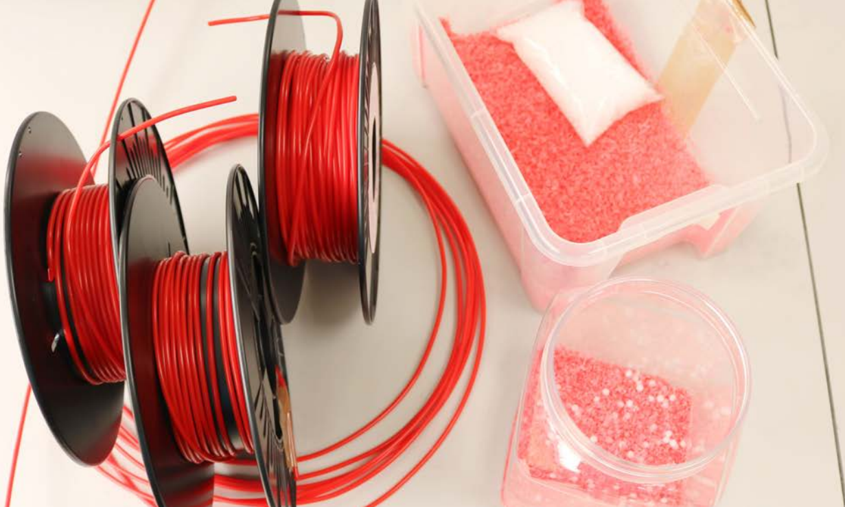
Figure 13 - Samples of recycled HDPE, and LLDPE regrind (before and after mixing)
