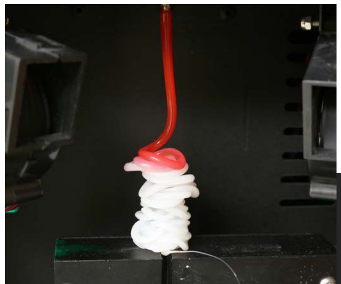
Figure 9 - Transition from HDPE (bottom) to shredded LLDPE (top)
