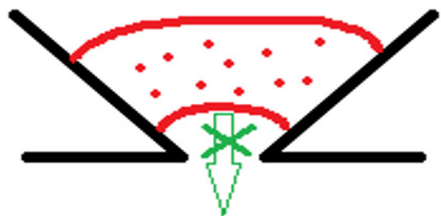
Figure 11 - Bridging : the material forms a cohesive structure against the walls of the hopper, making the feeding inconsistent
