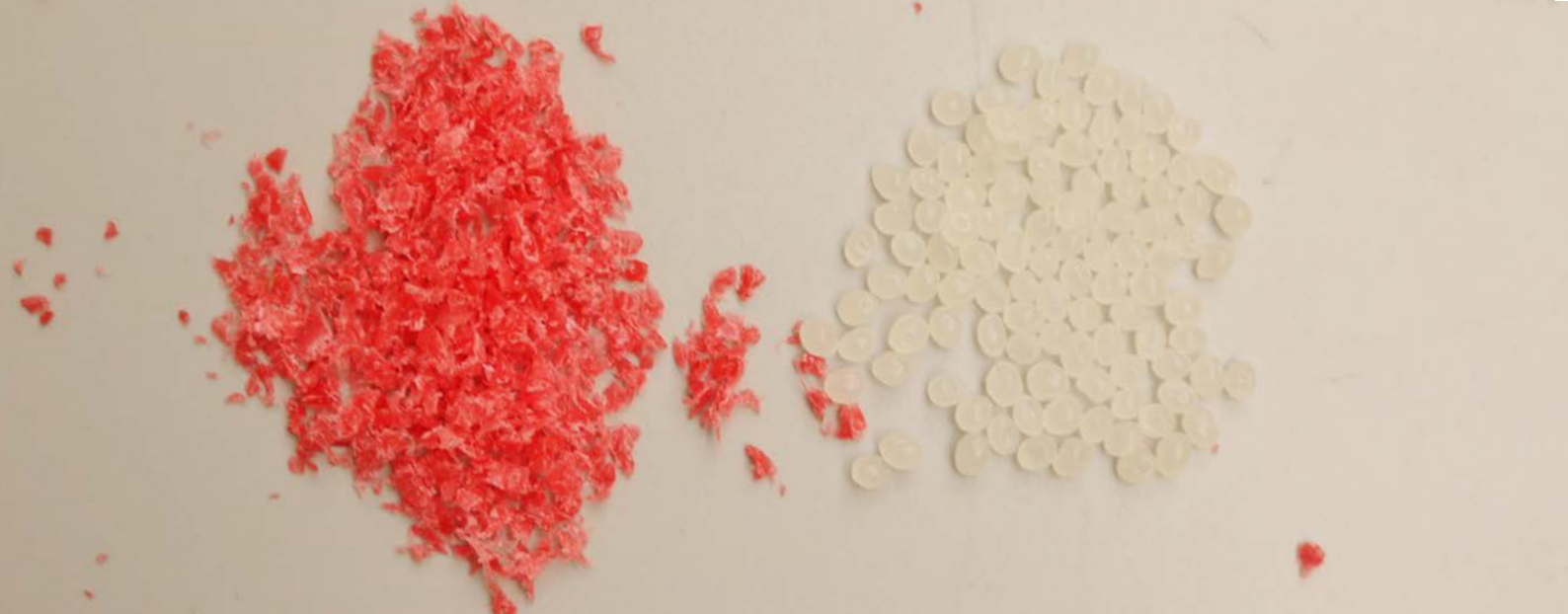
Figure 7 - Size and shape comparison between LLDPE regrind (left) and standard PLA pellets (right)
