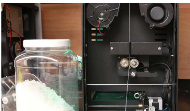
Figure 8 - Filament flowing freely during the adjustment phase, since the filament quality was not of sufficient quality yet to spool at this point
