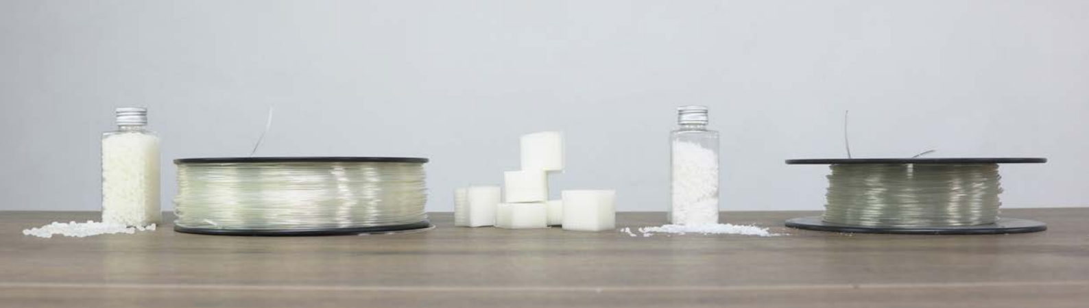
Figure 1 - Products within the recycling process (Virgin PLA > Filament > 3D-prints > Regrind > Filament)
