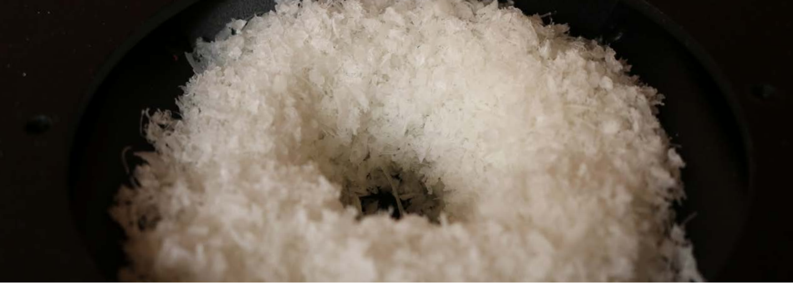
Figure 6 - Ratholing of PLA regrind in the machines' hopper
