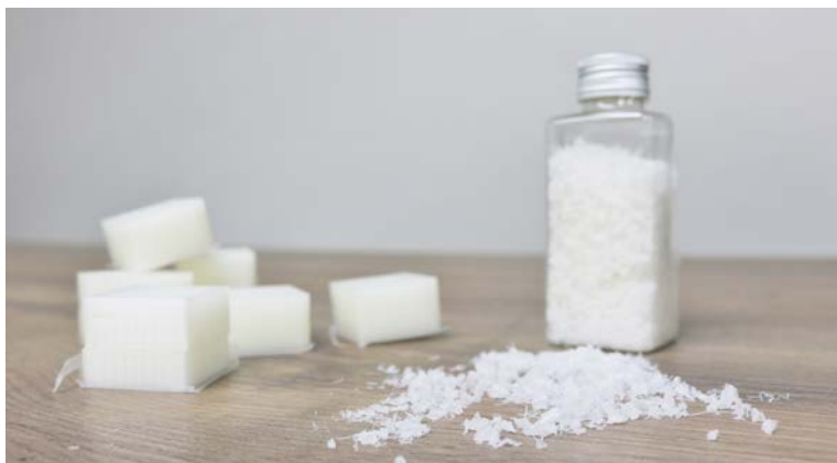
Figure 3 - The 3D-printed blocks and the resulting regrind after shredding
