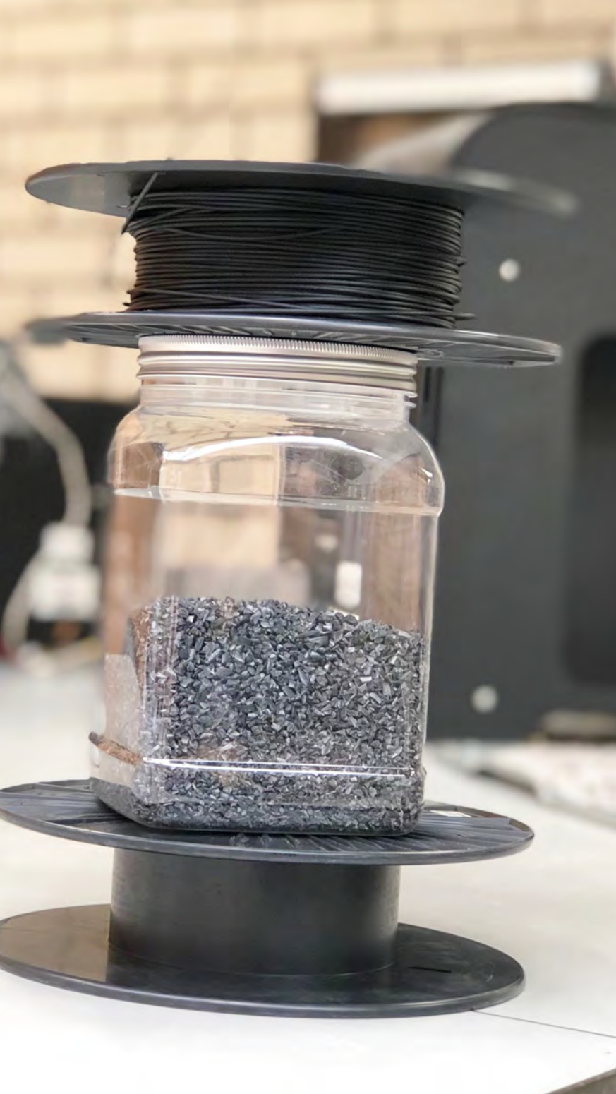
Figure 8 - Initial spool of PS (bottom), jar of PS regrind (center), spooled recycled PS
