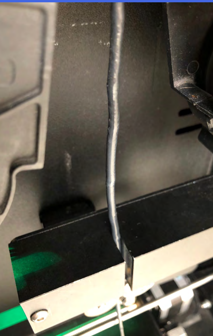
Figure 4 - First PS output obtained at high RPM (to speed up the transition process)
