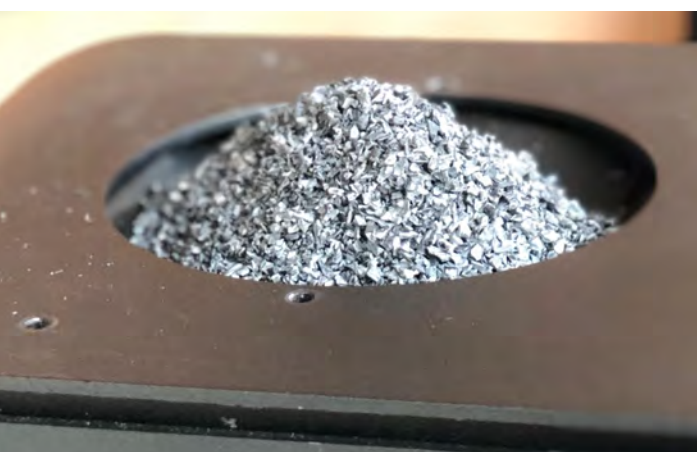
Figure 3 - Feeding PS into the hopper of the extruder
