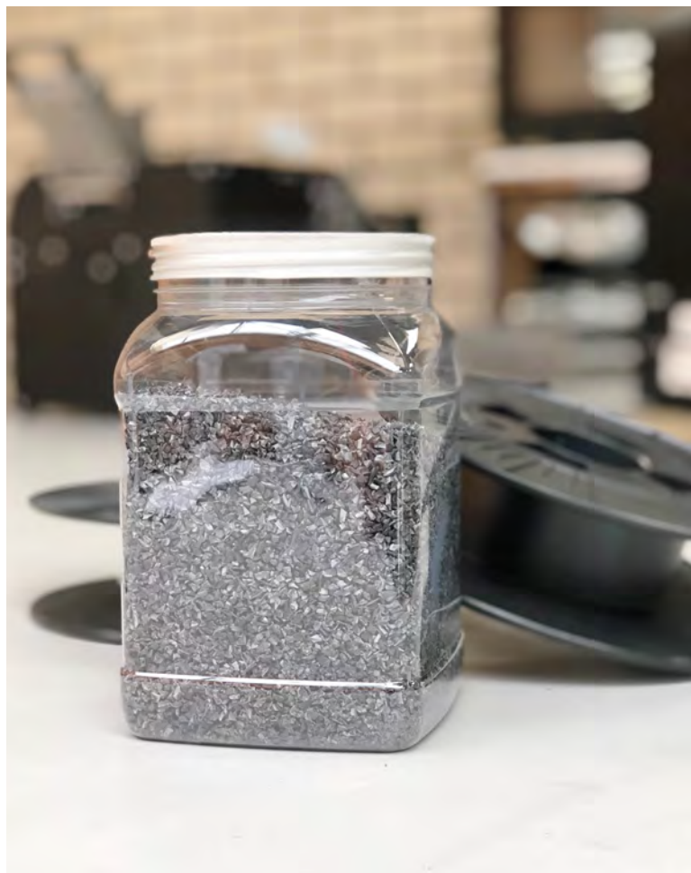
Figure 1 - PS regrind in the jar, original spools behind it
