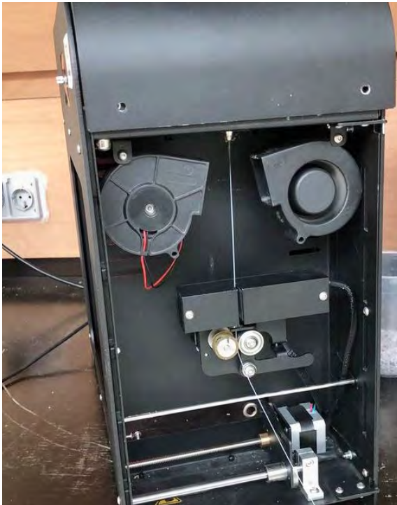
Figure 5 - Filament flowing freely during the adjustment phase
