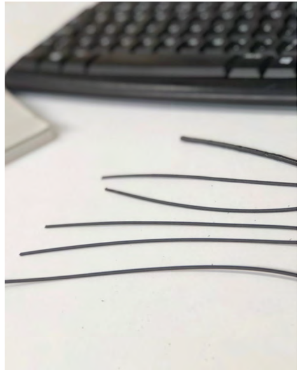
Figure 6 - Filament thickness controlled by the filament sensor: thinner and thinner down to the desired thickness (top to bottom)
