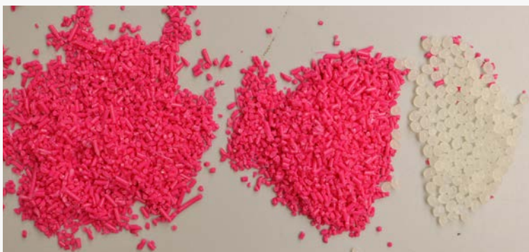
Figure 6 - Size and shape comparison between PLA regrind (left), PLA regrind after a second shredding step (center), and standard pellets (right)
