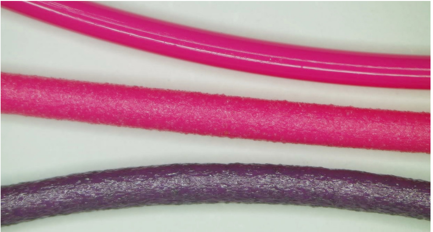
Figure 14 - Microscope shot of (top to bottom): recycled virgin PLA, recycled PLA+GP, recycled PLA+CF
