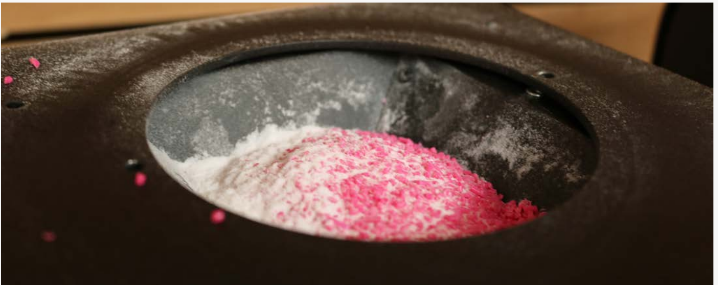
Figure 10 - Feeding the PLA+GP blend in the hopper of the extruder
