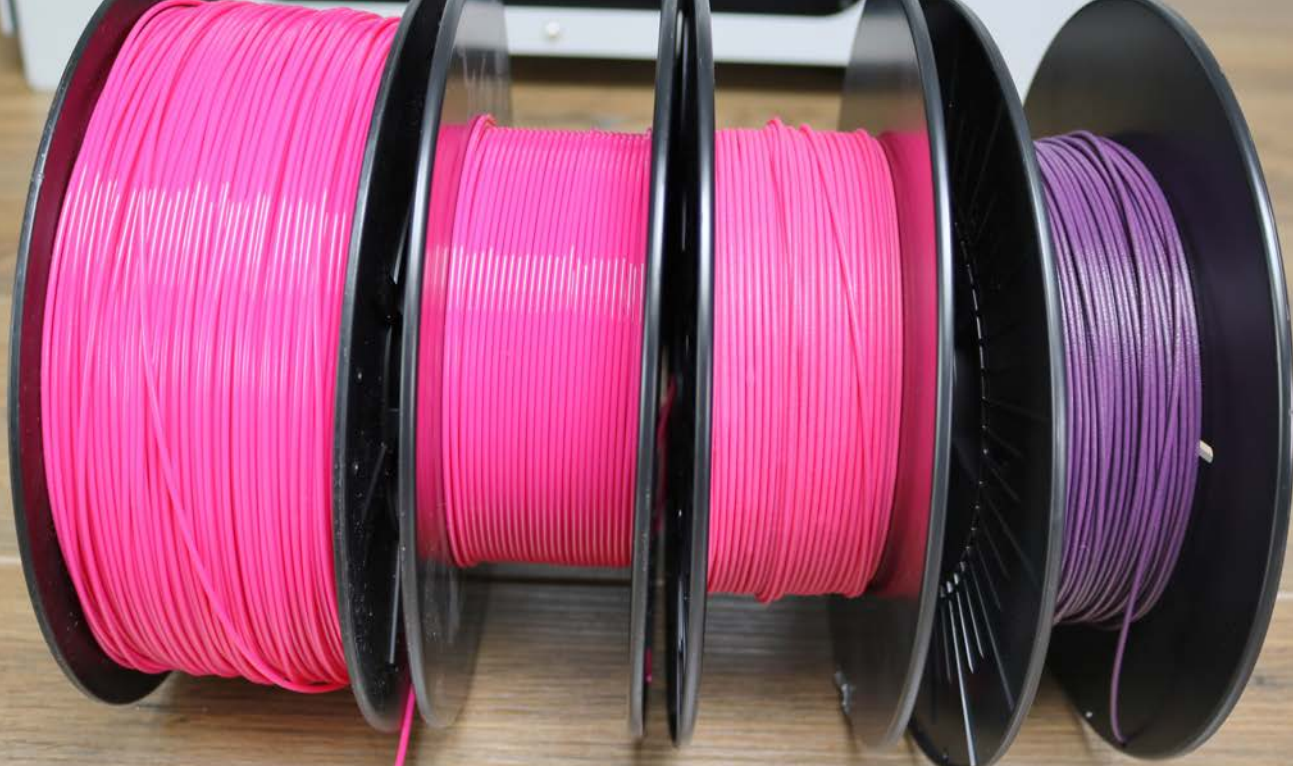
Figure 16 - Left to right: original spool of bq PLA 3D-printer filament, recycled virgin PLA filament, recycled GP-filled PLA filament, recycled CF-filled PLA filament
