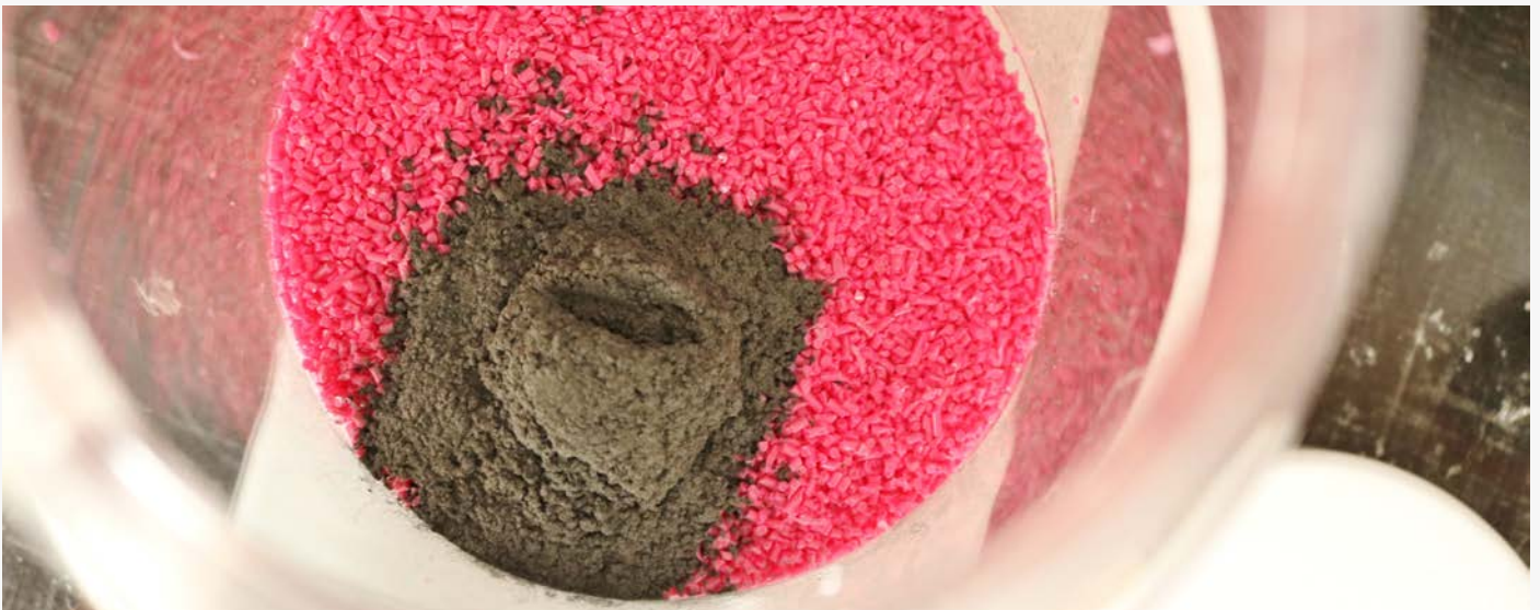
Figure 12 - PLA regrind and 3%w CF in a jar, before they were mixed
