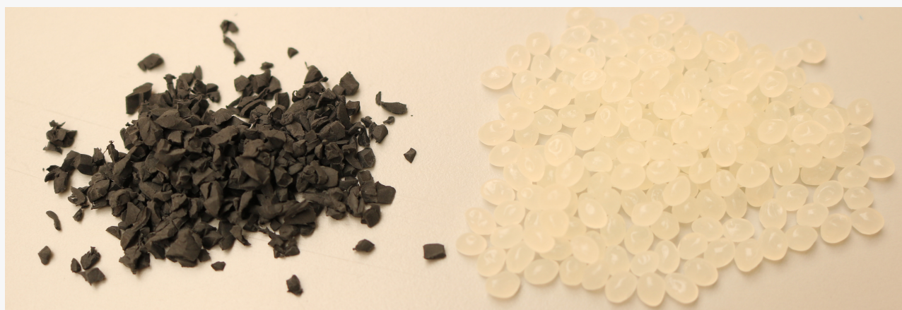
Figure 5 - Size and shape comparison between SEBS regrind (left) and standard PLA pellets (right)
