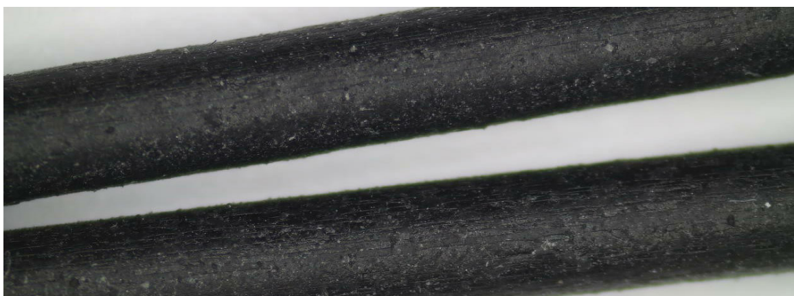
Figure 12 - Microscope shot, slight roughness on the surface of the filaments (recycled SEBS on the top, pristine SEBS on the bottom)
