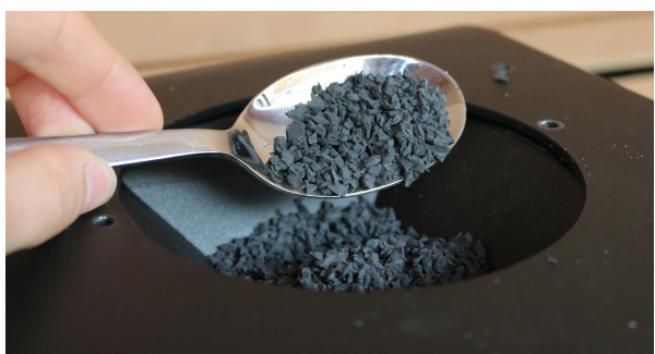
Figure 8 - Feeding SEBS regrind into the hopper of the extruder
