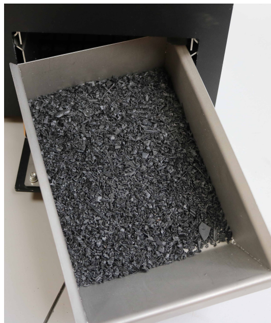
Figure 4 - First sample of regrind coming out of the SHR3D IT
