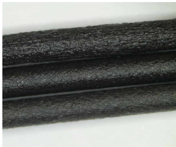
Figure 12 - Microscope shot to compare the visual aspect and roughness of each filament : (from top to bottom) recycled Onyx when extrusion temperatures are too high and/or when the material has not been dried prior to extrusion, recycled Onyx with the correct settings, commercial unrecycled Onyx filament
