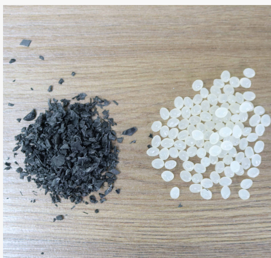
Figure 5 - Size and shape comparison between Onyx regrind (left) and standard PLA pellets (right)
