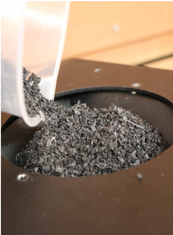
Figure 8 - Feeding Onyx regrind into the hopper of the extruder
