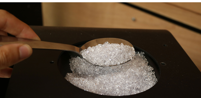
Figure 3 - Feeding PETG into the hopper of the extruder
