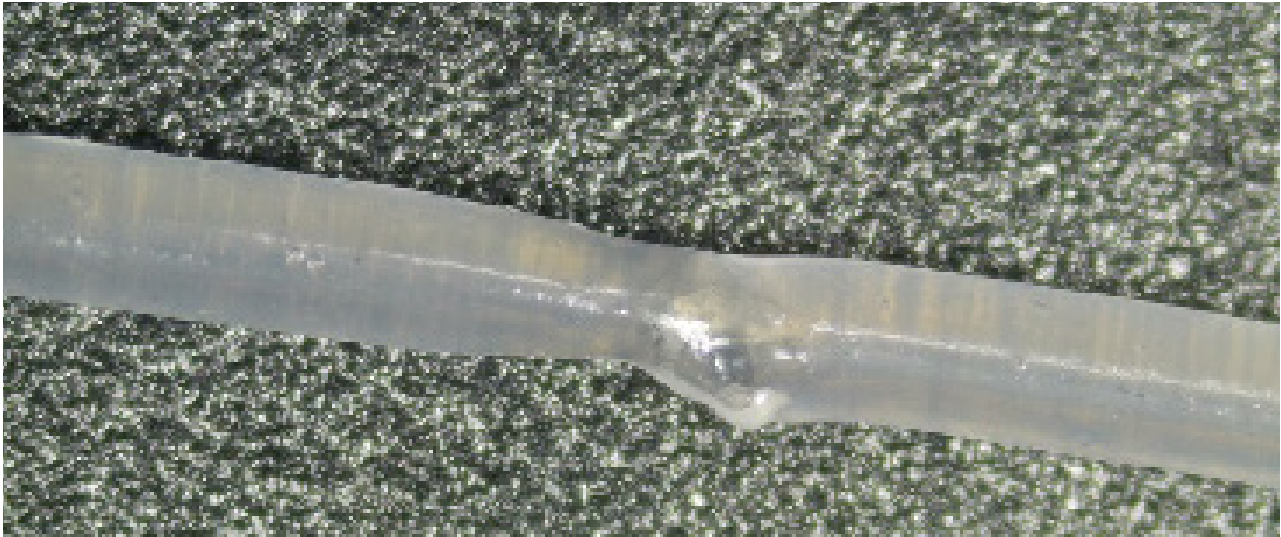
Figure 14 - Microscope shot: view of the filament when temperatures were set too low
