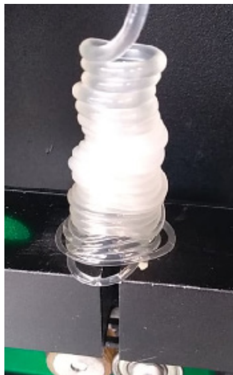
Figure 9 - Transition between purging PLA (transparent extrudate at the bottom) and PP (semi white and opaque extrudate above PLA)
