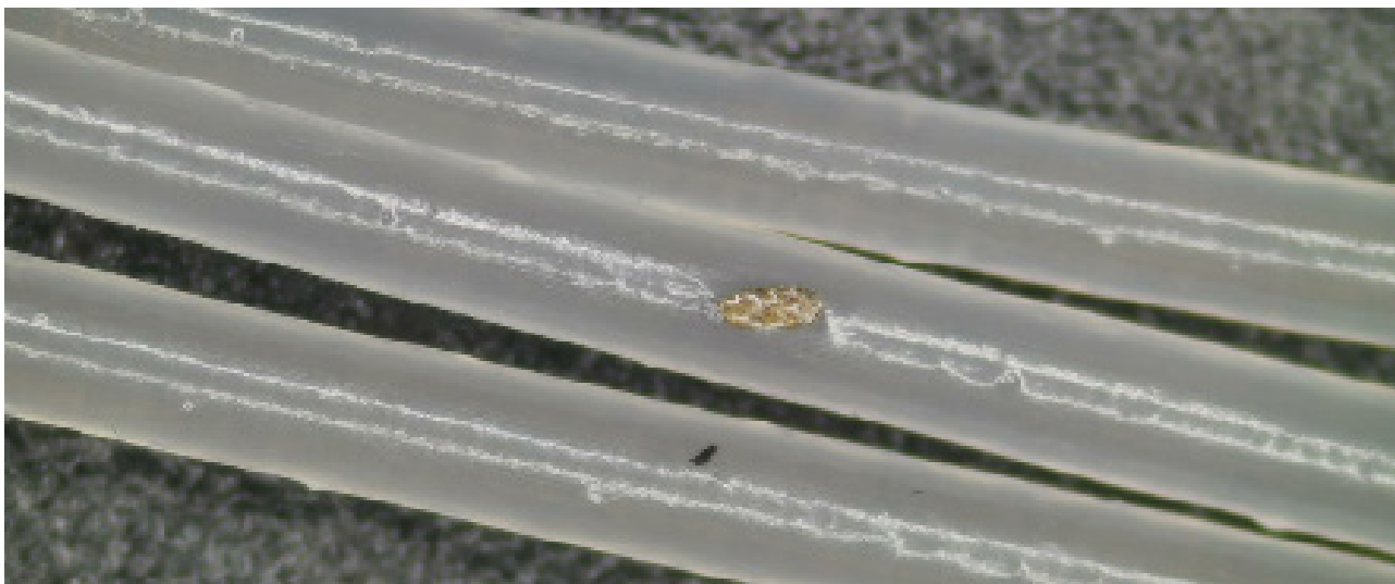
Figure 15 - Microscope shot: view of the filament of good quality, only the dust remains
