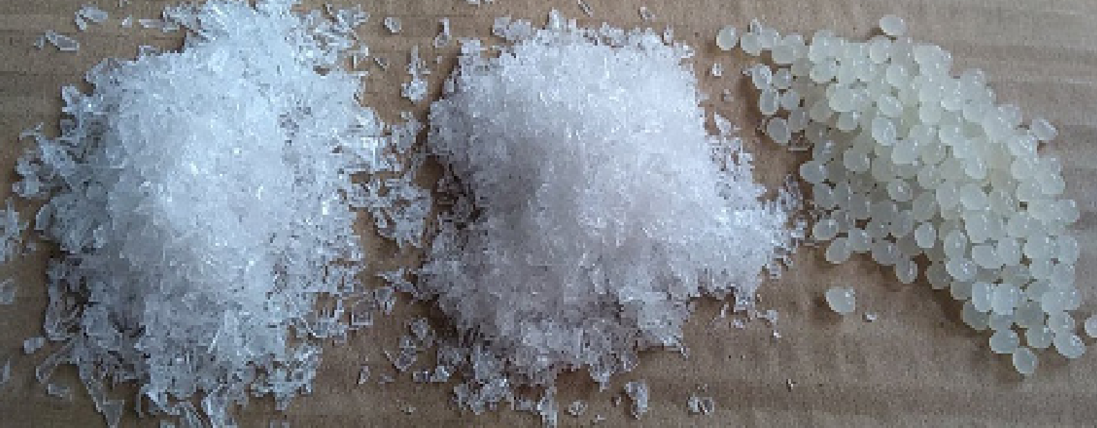
Figure 7 - Size and shape comparison between regrind (left), second regrind (center), standard PLA pellets (right)
