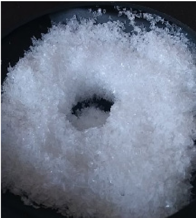
Figure 10 - Rat holing occurring in the hopper
