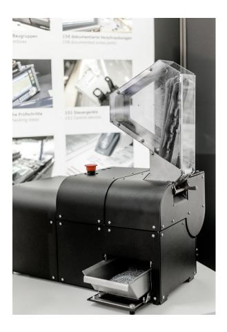
The Shr3d It could shred the plastics into small, processable and extrudable pieces with precision – an important requirement for preventing lumps in the final filament.
